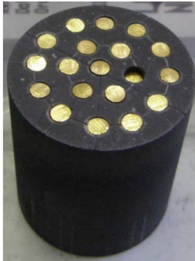
Figure 8. The example of design of a cylindrical cathode of main discharge, containing cylindrical rods from different materials, for instance, silver, tungsten, gold etc. This is item 1 n Figure 7, [8].
