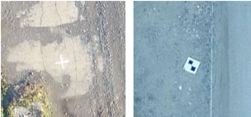
Figure 5. (Ground) control points; left - marking using a spray; right - using black-and-white target
