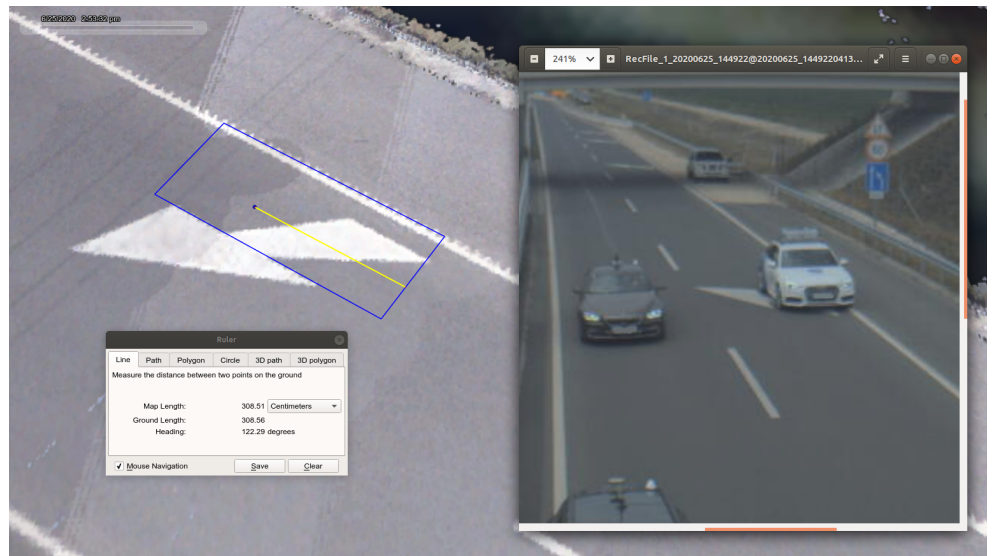
Figure 29. Outlines of white-blue Audi based on position data, plotted on UHD map of M86 section. The image was taken at the same moment. The position of the Audi on the image corresponds with the plotted outlines.
