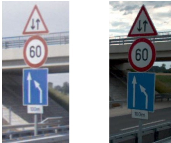
Figure 8. Shooting from the same spot (left: Leica Pegasus 2 Ultimate 360° panoramic photo crop, right: Ladybug 5+ (Riegl) Camera Picture crop)
