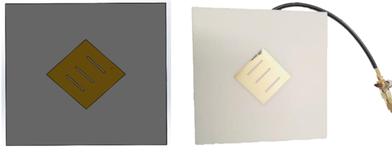
Figure 4: (left) IGLUNA 2020 slotted patch antenna (reference antenna) CAD design; (right) prototyped hardware
