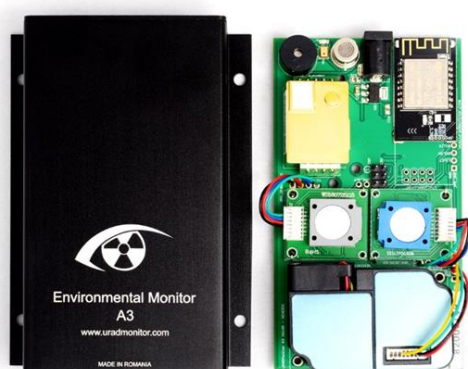
Figure S1. uRAD A3 air quality monitor hardware [15].
