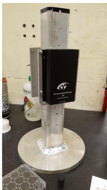
Figure S2. A3 monitor fixed onto the aluminium stand.
