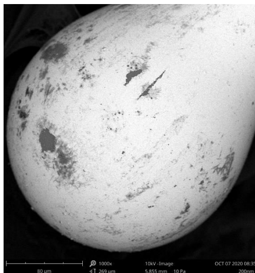
Figure 1. SEM image of the microsphere-sensor with a 100 nm ZnO ALD coating. Magnification of 1000x.
