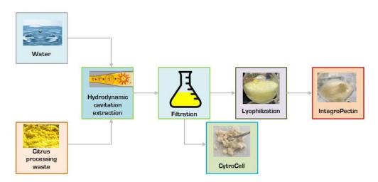
Scheme 1. Biorefinery scheme for citrus processing waste based on hydrodynamic cavitation.
