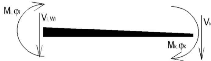
Figure 9 Sign conventions for moments, shear forces, displacements, and slopes for stiffness matrix
