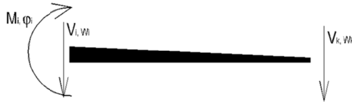
Figure 11 Sign conventions for moments, shear forces, displacements, and slope for stiffness matrix
