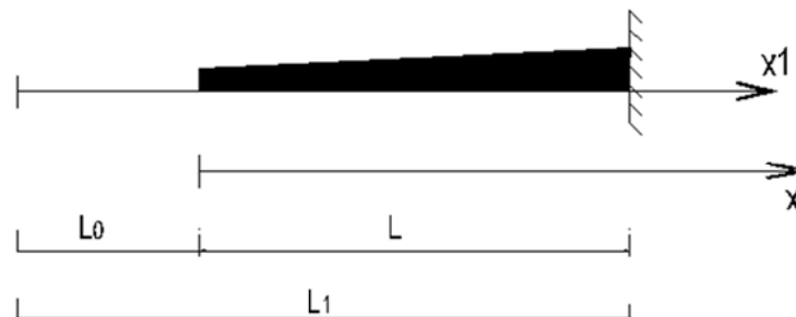
Figure 24 Vibration analysis of a tapered free–fixed beam
