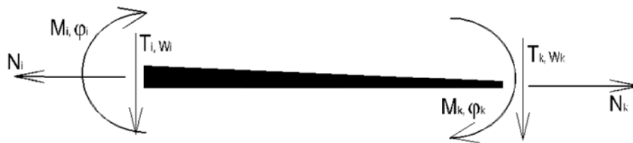
Figure 13 Sign conventions for moments, transversal forces, displacements, and slopes for stiffness matrix
