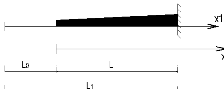
Figure 24. Vibration analysis of a tapered free–fixed beam.
