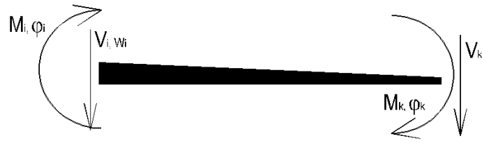
Figure 9. Sign conventions for moments, shear forces, displacements, and slopes for stiffness matrix.
