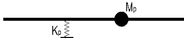
Figure 14. Vibration of beam having a concentrated mass and a spring.
