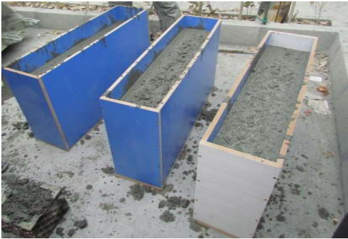
Figure 4. Casting by concrete of three deep beam.
