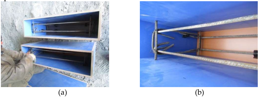
Figure 3. Detail of bars and three deep beams (a) Frameworks and (b) Bars inside the framework.
