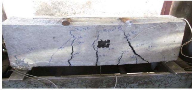
Figure 10. Crack path observed by experimental test (B-0).
