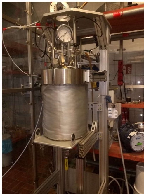
Figure 1. View of pilot scale stirred tank stainless steel reactor of 18.875 L (Parr, USA, Model: 4555).
