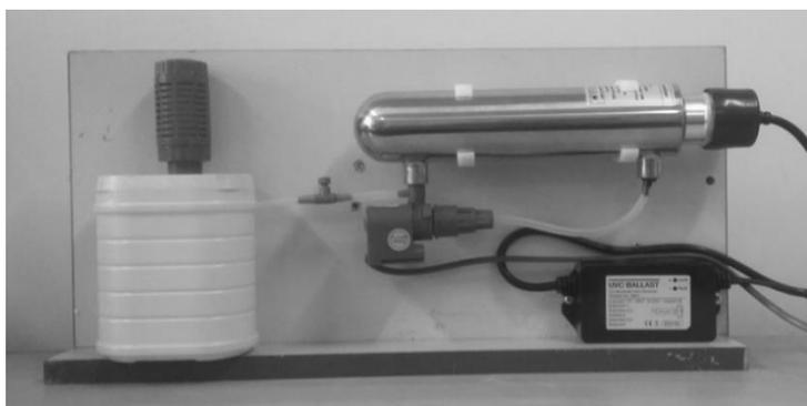
**Figure 2.** Lab-installed UV disinfection unit
