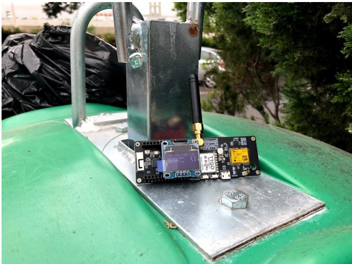
Figure 15. LoRa probe installed on top of an Iglô.
