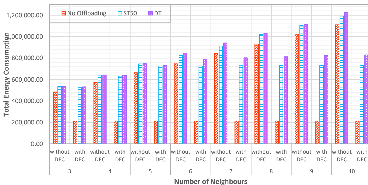
Figure 12: impact of increasing number of neighbours on Energy consumption with various offloading schemes
