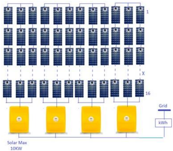
Fig. 5. Schematic block diagram of the PV system.
