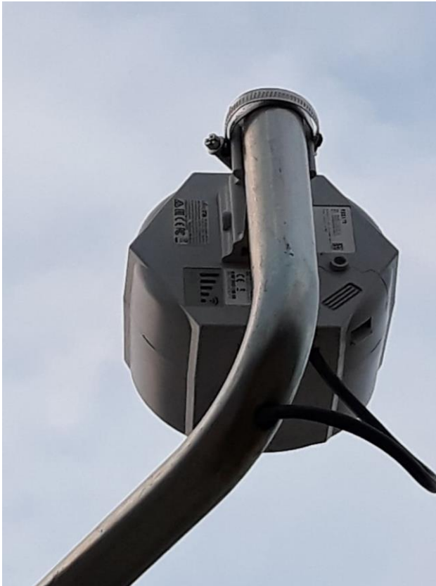
Fig.11: 10-dbi directive Mikrotik antenna to increase the 4G signal level. I+D Energías, Poland
