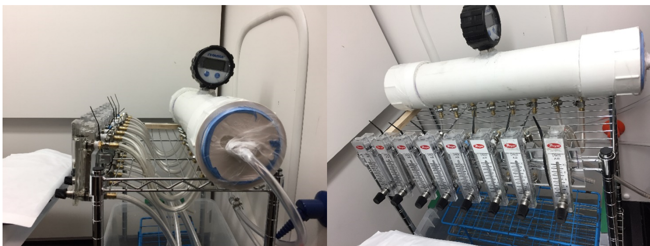
Supplementary Figure 10. Visual verification of air flowrate in each treatment (II). Eight Dwyer flowmeters were mounted on a stainless-steel shelf so that they can be positioned vertically to ensure accurate readings. A digital pressure gauge (range -15 psi to 15 psi, \pm 0.5\% full scale) (DPG108-015CG, Omega Engineering Inc., Stamford, CT 06907) was installed on top of Manifold 2. The same installation procedure was followed as for other sensors and gauges.
