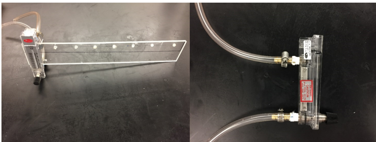
Supplementary Figure 9. Visual verification of air flowrate in each treatment (I). An acrylic board was cut, and eight holes were drilled on it so that the rotameters (RMA-21-SSV, Dywer Inc. Michigan City, IN, USA) can be mounted on it.
