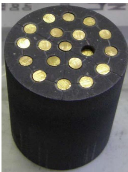
Figure 4. The example of design of a cylindrical cathode of main discharge, containing cylindrical rods from different materials, for instance, silver, tungsten, gold etc. This is item 1 in Figure 3, [11].
