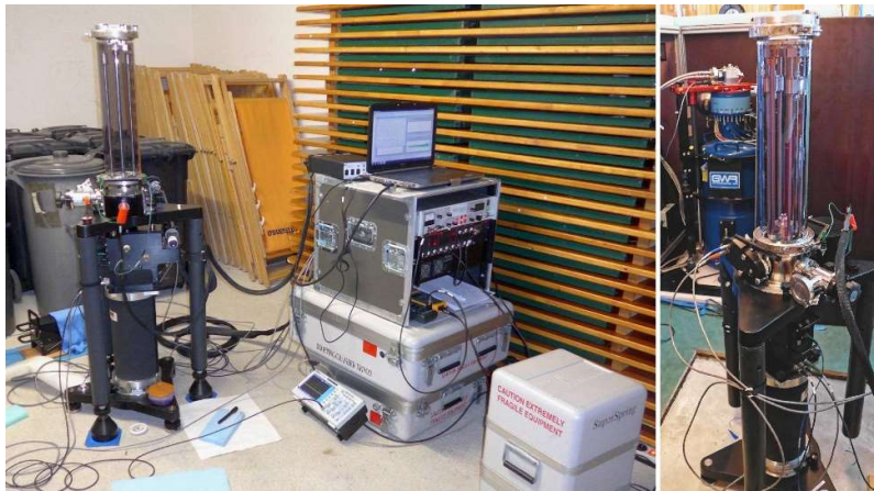
Figure 3. (left) Absolute gravimeter FG5X-220 with control electronics at the site Wank Berg in 2019; (right) FG5X-220 operating close to the superconducting gravimeter OSG#052 at Zugspitze.
