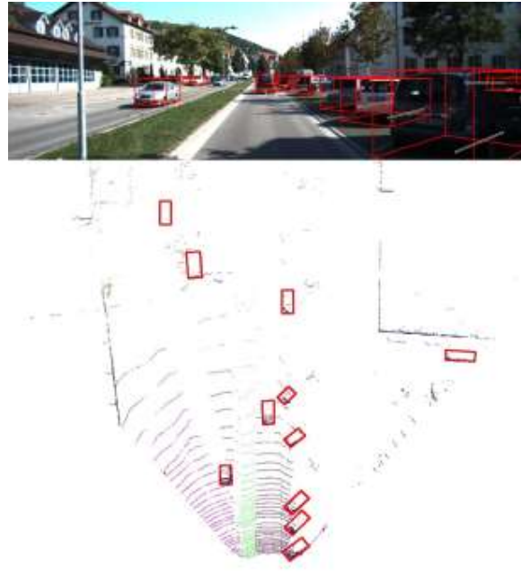
Figure 15. LiDAR's bird eye view plus boxing object detection [60].
