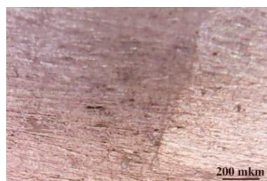
Figure 1. Optical microscopy (magnification x500) varnish / xylene / filler KPT-8: 10/10/1 film.
