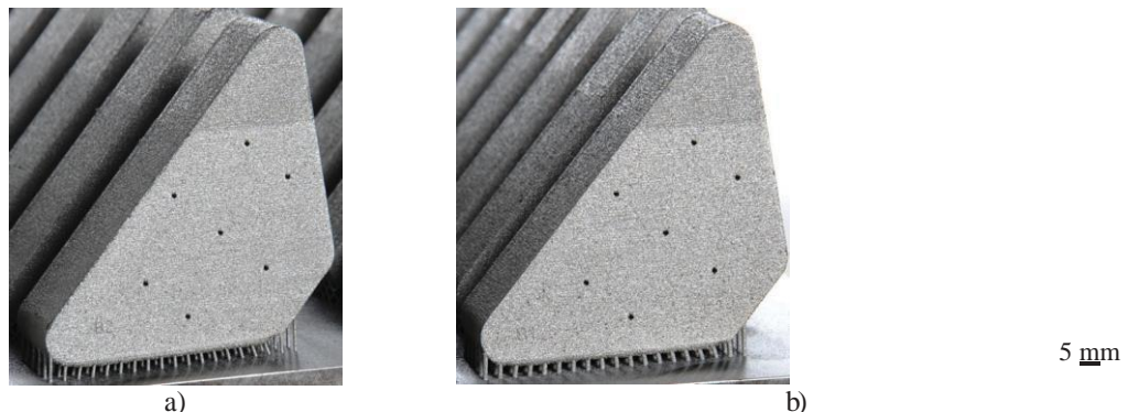
Fig. 7 Deflections of the bar support structures with a strut diameter of: a) 0.7 mm, b) 1 mm
