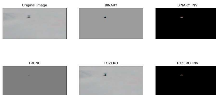
Fig. 2 results in photo processing by Thresholding function OpenCV
