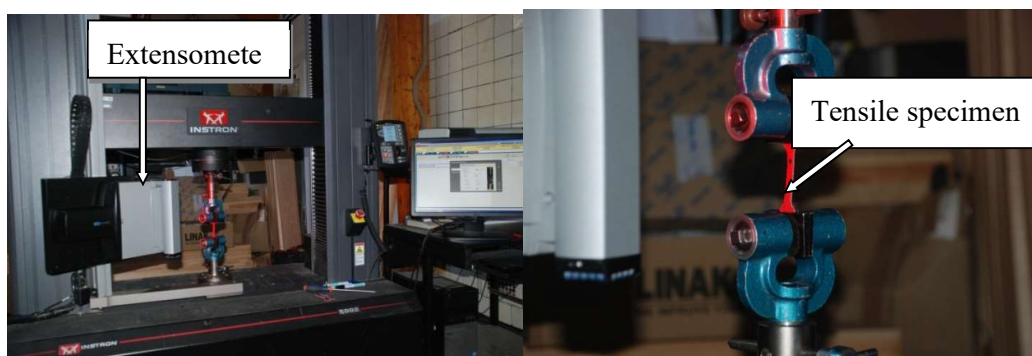
Figure 2. An uniaxial tensile specimen mounted on the testing machine.
