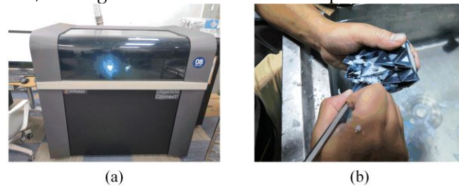
Figure 4. Waterbomb thin-shell structure fabrication: (a) 3D printing and (b) support material removal
