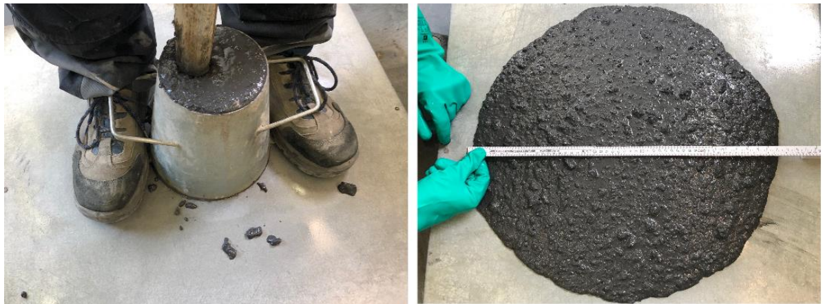
Figure 2. G50M33R17-11 during workability test
