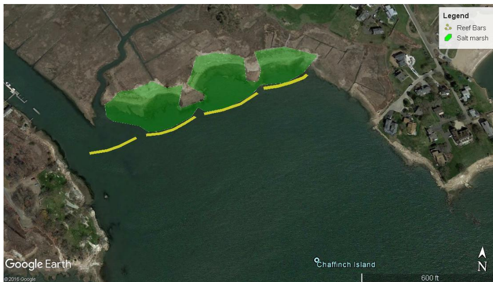
Figure 22: Proposed resilience plan for protecting the coastline, Yellow lines: reef balls, Green polygon: salt marsh. This is just a fundamental plan. To have a sustainable and resilient protection system and ensure accretion rates of salt marsh, a comprehensive study should be done on sediment supply from West River and circulation in the coastline. The system should be able to accumulate sediment supplies from the West River.
