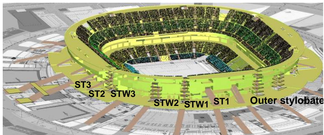
Figure 11. 3D model of the Gazprom Arena stadium (northeastern view) built in the Sigma PB software and seating in the stands.
