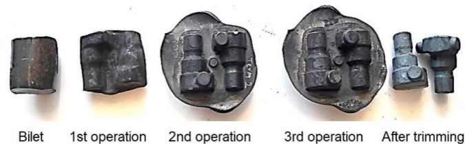
Fig. 2. View of a forging in particular operations
