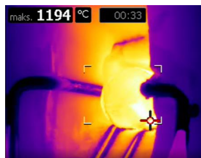
Fig. 3. Measurement of the preform temperature at the point of removal from the heater
