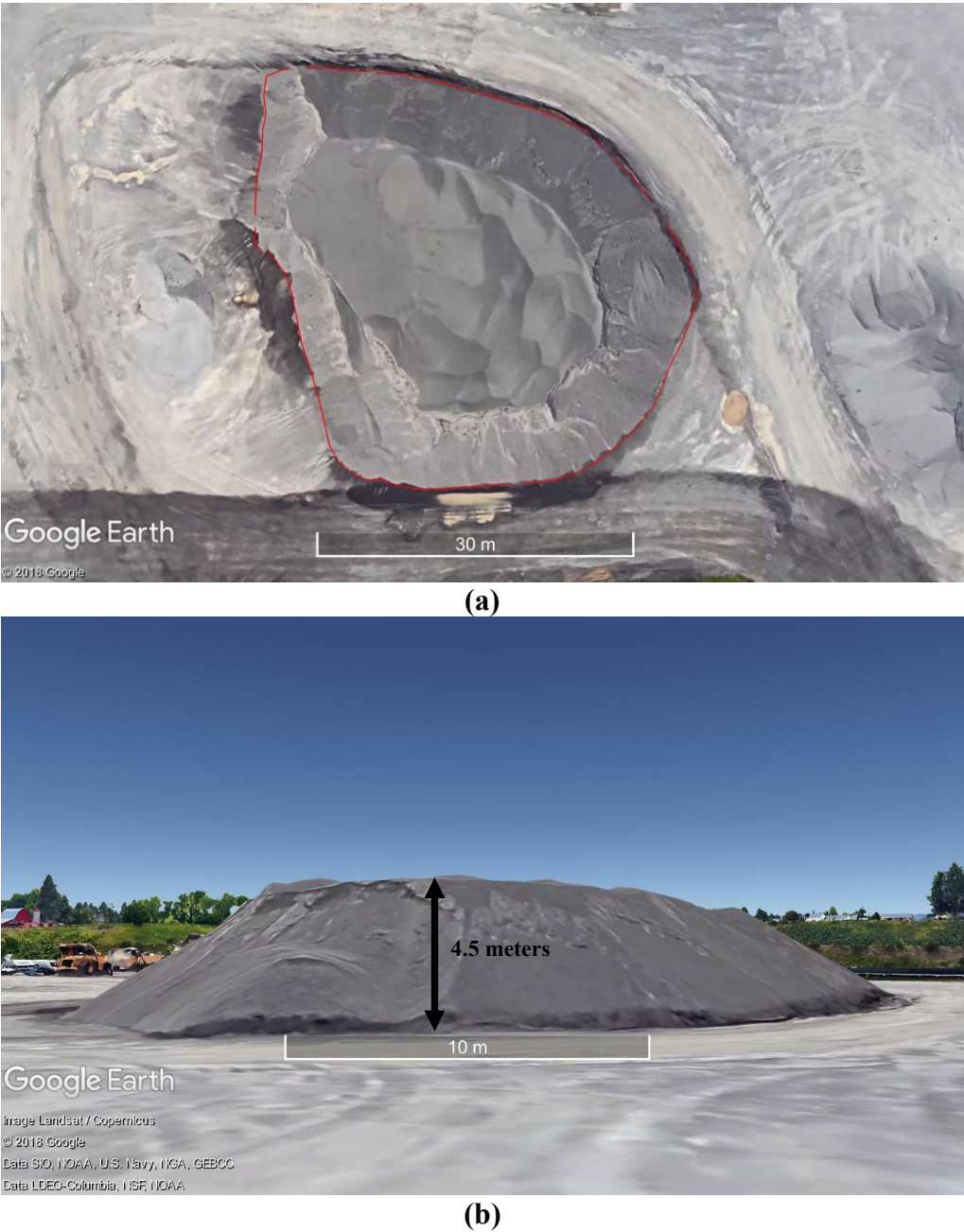
Fig. 2. A sample 3D rendering of an aggregate stockpile in Google Earth, a) in aerial and b) oblique view, showing approximate height.
