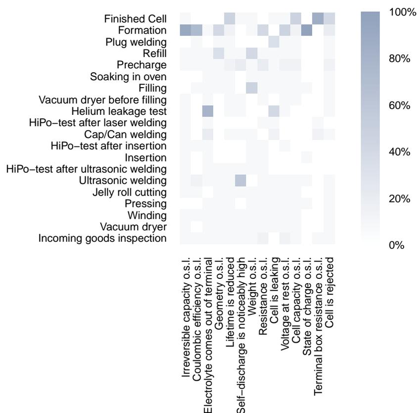
**Figure 7.** Possible relative reduction of failure rate for several final product characteristics given that a certain process runs failure-free. (o.s.l. = outside the specification limits)
