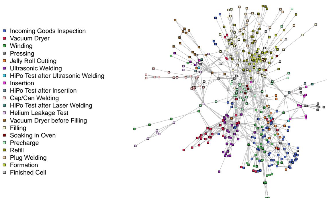
**Figure 5.** Failure network where each node is a failure color-coded in its corresponding process step (legend of process steps sorted in chronological production process order starting from the top)
