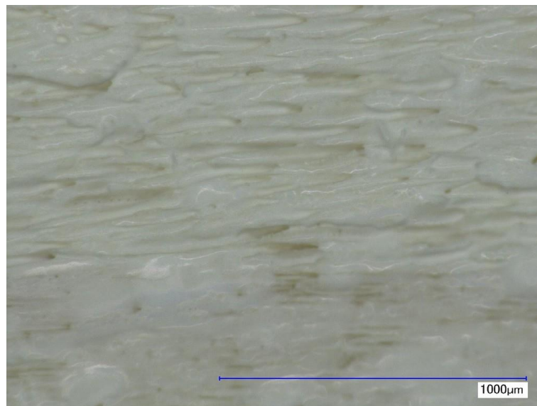
Figure 1. Light microscopic image of the PS sphere coated pine wood sample.
