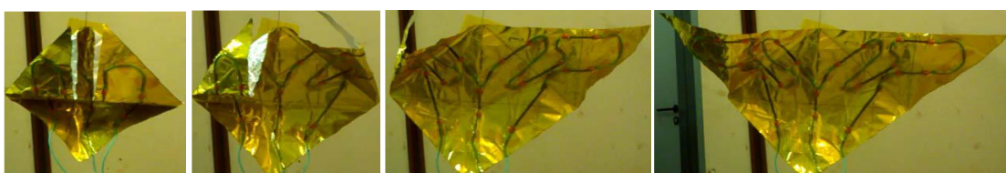
Figure 7. Sail prototypes configurations 1-5 with SMA elements; length of SMA elements: 5 cm, 4 cm, 3.5 cm, 3 cm, 2.5 cm, 2 cm.
