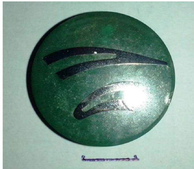
Figure 8. Metallographic specimen of material of the LPT blade.
