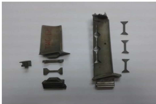
Figure 7. View of specimens cut out, by using the electro-discharge method, of a material of the LPT blade and view of specimens for static tensile testing, cut out of material of HPT blade and LPT blade.
