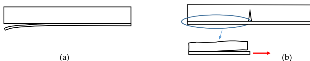
Figure 10. Debonding mechanisms: (a) end debonding, (b) intermediate crack debonding.
