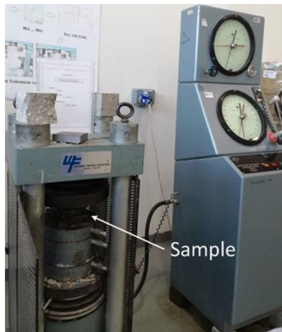
Figure 3. Set-up of compressive strength showing the placement of the specimen.
