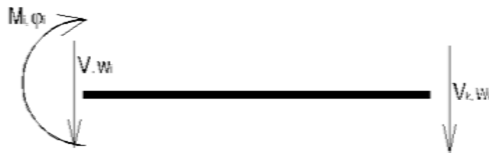
Figure 3. Sign conventions for moments, shear forces, displacements, and rotations for stiffness matrix
