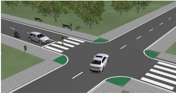
(c) Time Frame 2 - Vehicle 1 starts moving to left toward the zebra crossing while vehicle 3 is standing still. The pedestrian 1 is in the middle of the zebra crossing and pedestrian 2 is standing still.
