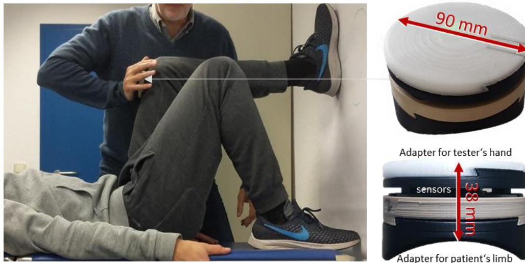
Figure 1. Setting of MMT of the hip flexors with fixed leg including the handheld device. The assistant's leg is fixed against the wall to ensure a stable position also after repeated trials. The tester's forearm is in rectangular position to the rectus femoris muscle. The handheld device is located between the tester's hand and the assistant's distal thigh to measure the force profile produced by the tester. On the right side, the handheld device with two adapters is illustrated: one for the palm of the tester (white) and one for the limb of the patient (black), which is shaped according to the contours of the limb. Between the adapters, the sensor technology is placed. Dimensions of the handheld device are given in mm.
