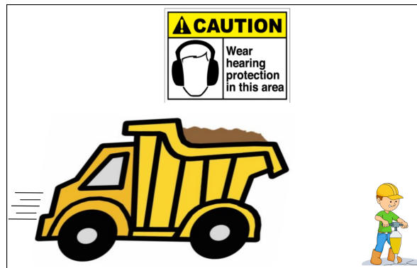
Figure 1. Unaware worker in blind spot of a reversing dumper
