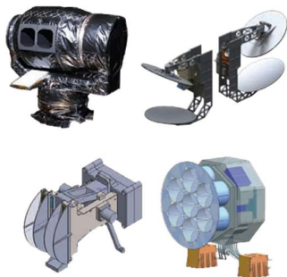
Figure 1 AMCS Thermal-IR Sounder Overview (Top Left), WAVE Sub-mm Sounder Overview (Top Right), MAVRIC Camera Overview (Bottom Left), CROME Instrument Overview (Bottom Right)
