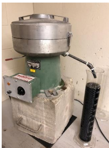
Figure 3. Centrifuge extraction apparatus: extraction of asphalt-solvent solution
