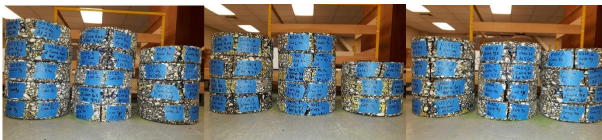
Figure 1. The 38 investigated HMA pavement core samples
