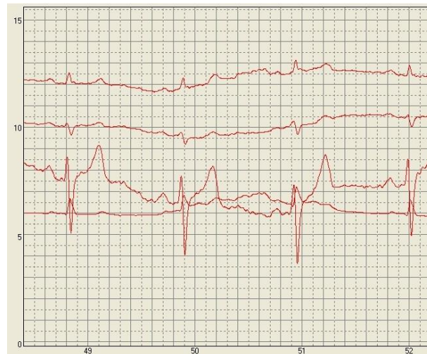
Figure 12. 4 ECG channels recorded through a layer of clothing using 4 textile electrodes of a large area and a compensating electrode connected to the human skin
