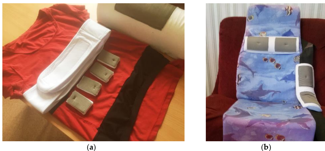
Figure 1. Electrodes made of conductive fabric embedded in clothes (a), in chairs (b)
