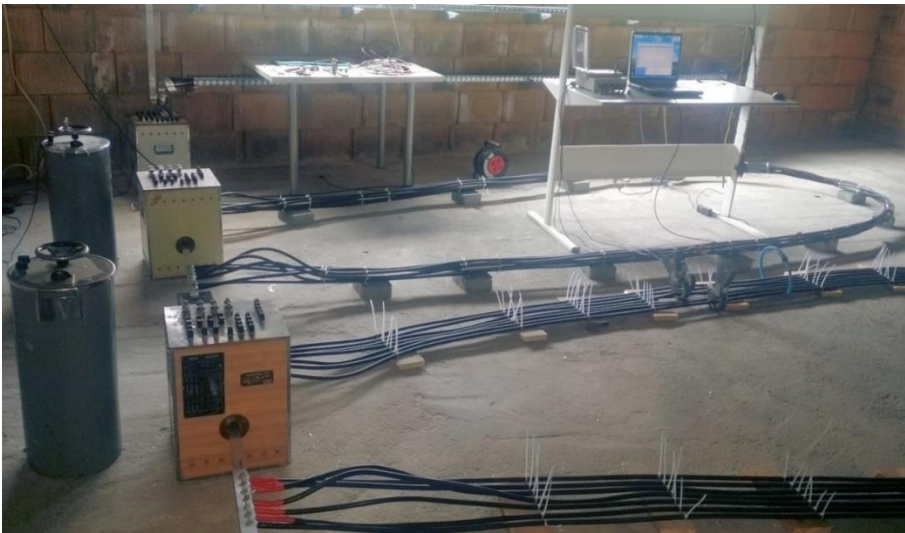
Figure 2. A photograph of the laboratory setup for examination of current distribution in the flat setup
