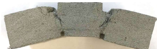
Figure 12. Flexural failure in an unconfined specimen tested under quasi-static shear loading.
