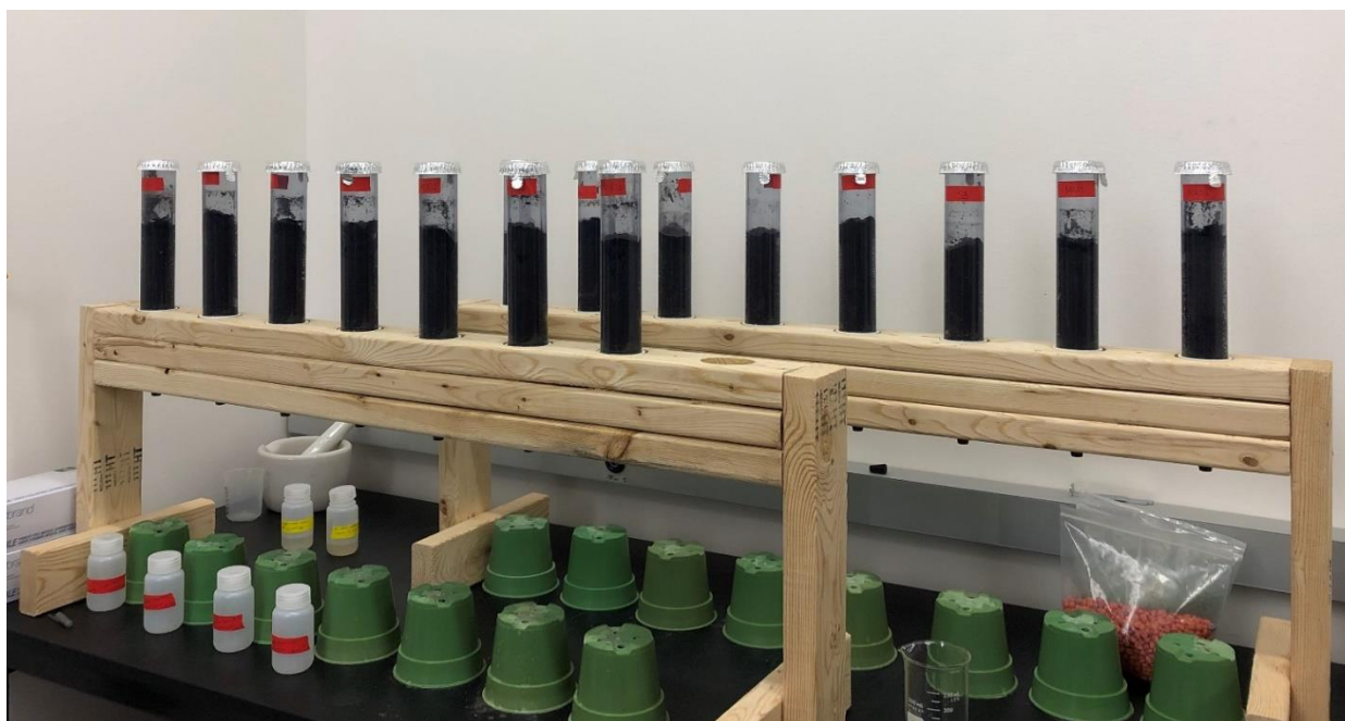
Supplementary Figure 1. A photo of the 15 soil columns on the wooden rack for the leachate collection. Each column contains 250 g of soil, treated with one of five treatments. Two of these apparatuses were utilized, resulting in 15 columns; three trials for each of the five treatments). M =manure control; S = soil control; MRO = manure and red oak biochar; MHAP = manure and highly alkaline porous biochar; MHAP-E = manure and highly alkaline porous engineered biochar.
