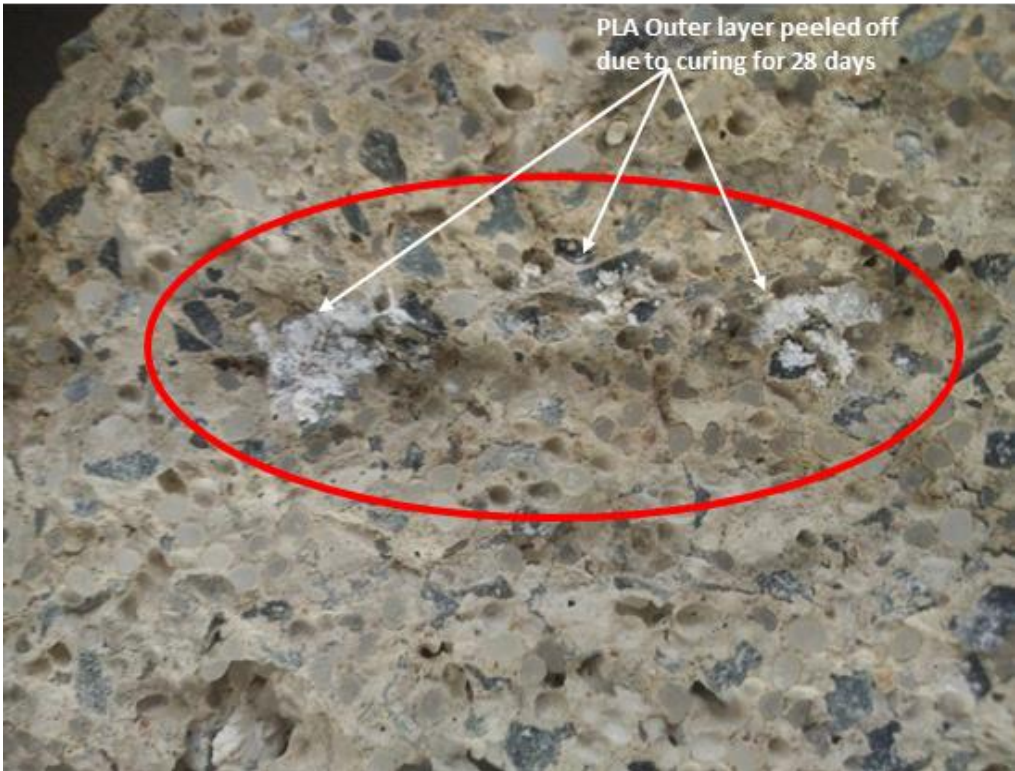
Fig 4. PLA outer layer (wafer or diaphragm) formed during curing period.
