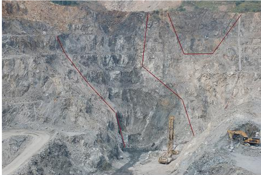
Fig. 3. Mining section with position of the ore body (black rocks) marked with red lines (view towards NW, photo 2014).
