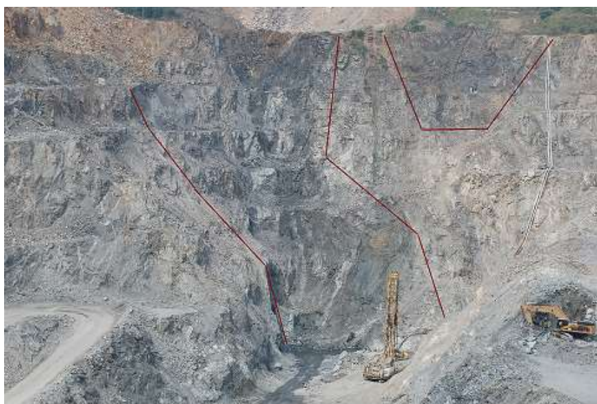
Fig. 3. Cross section through the deposit. Black rocks formed ore body marked with red lines (view towards NW, photo 2014).
