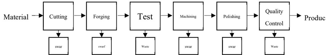
**Figure 3.** MEFCA structure for turbine blade production with the forging method.
